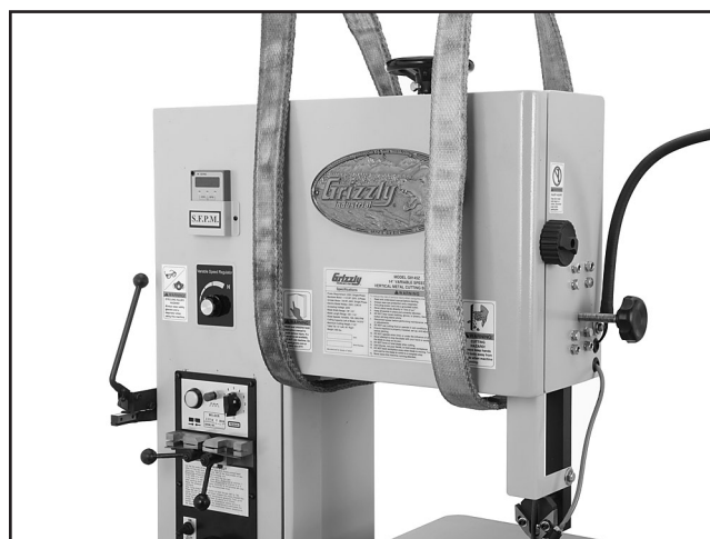
Figure 7. Lifting straps positioned on bandsaw.
